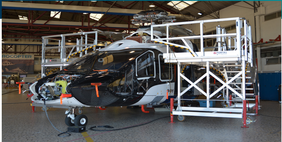
Figure 1: The pilot project is aimed at validating the simulation approach in the H160 in order to reduce the fuel system test cycles by a factor of two for the next helicopter models..
