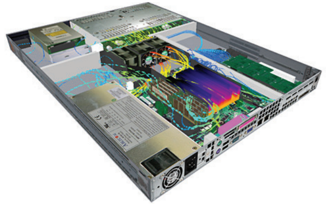
Figure 1. Airflow distribution in a 1U server modeled in Simcenter Flotherm.
